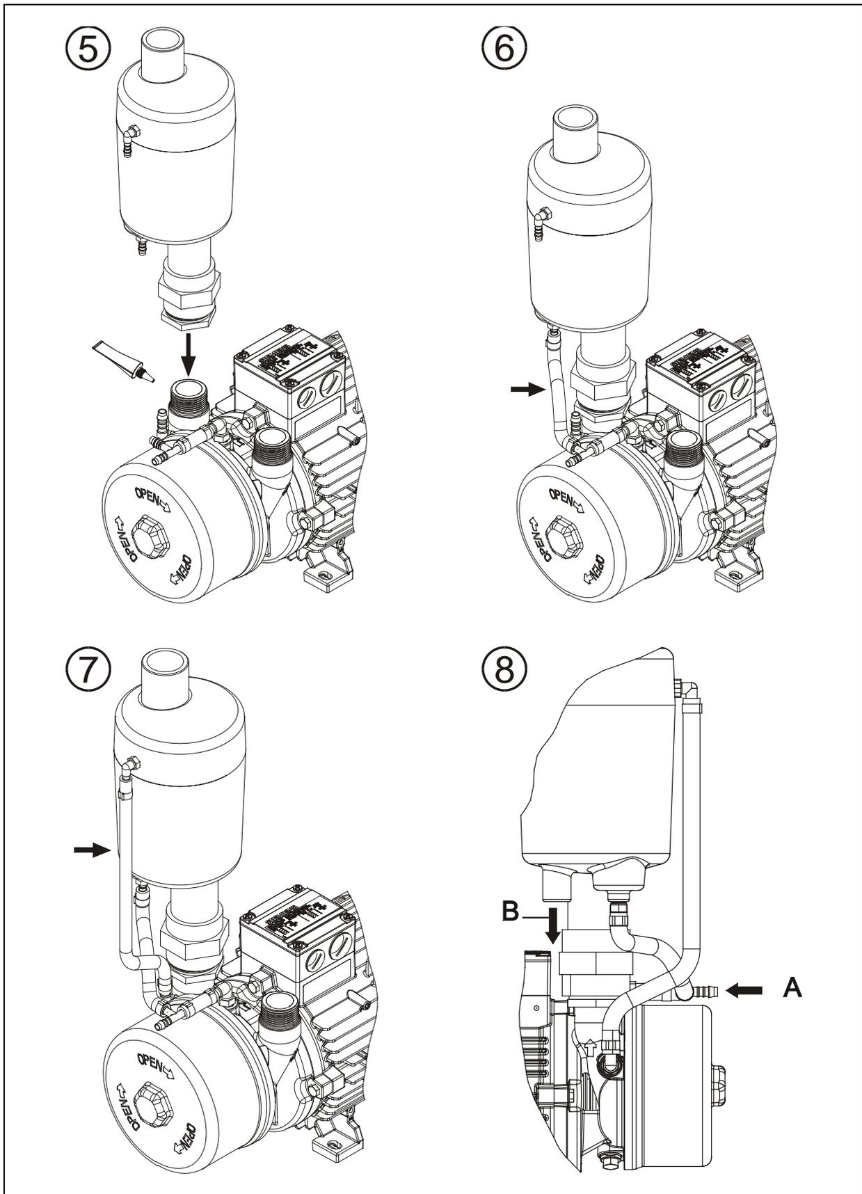
Fig. 21: Mounting liquid separator, Part 2 of 2
