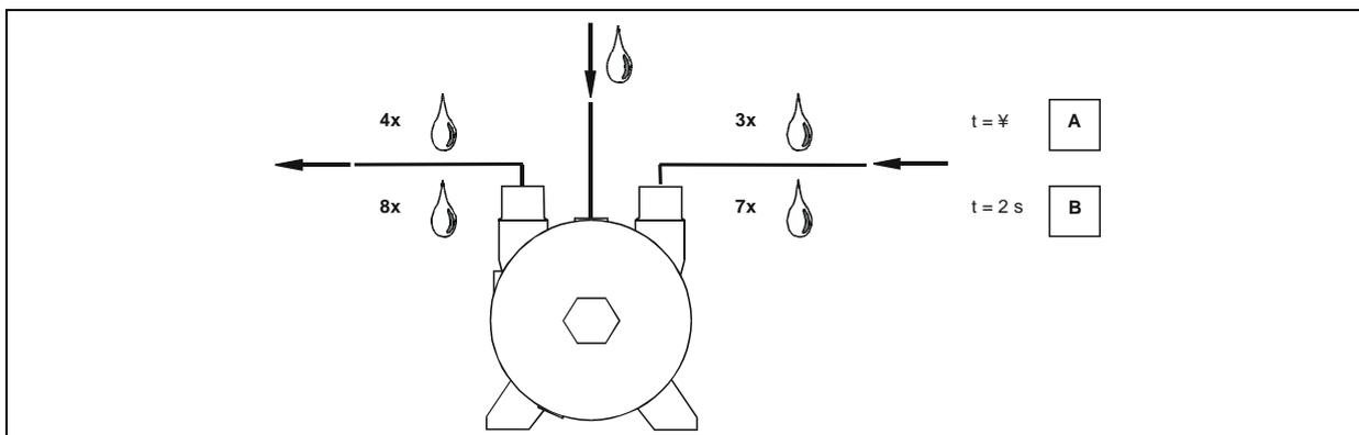
**Fig. 13: Maximum permissible quantity of water entrained via the inlet connection**
