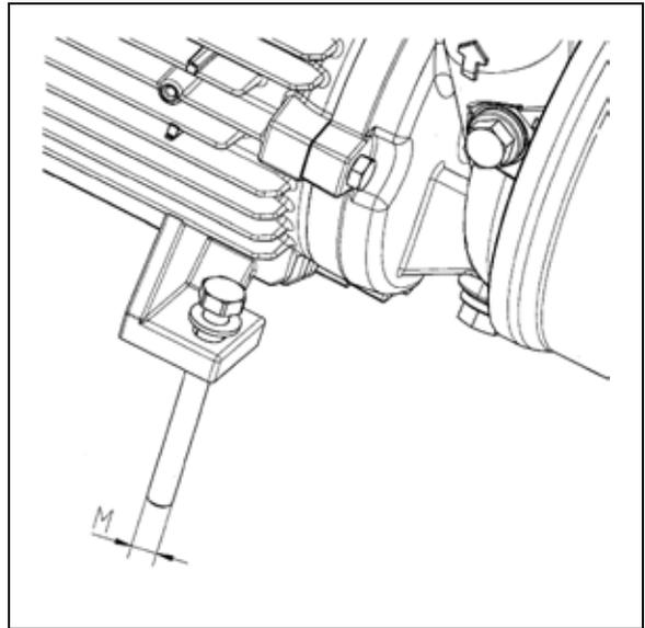
**Fig. 6: Securing elements for bolting feet to supporting surface**
