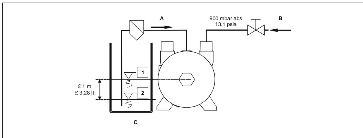
**Fig. 8: Self-priming operation**
