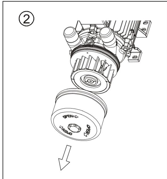
**Fig. 15: Removing vacuum pump/compressor housing**
