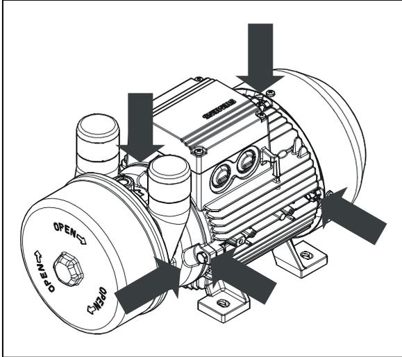
**Fig. 5: Points for measuring the vibration speed**
