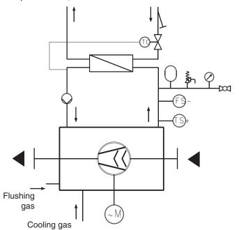
**Water-water radiator:** The external cooling circuit is connected to the factory's main water supply. It is equipped with a dust trap and a temperature controlled valve. This valve remains closed during the start run of the pump.
