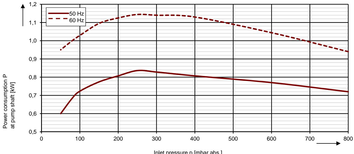
The characteristic curves are based on the evacuation of dry air and an intake temperature of 20 °C. At a suction pressure of 1013 mbar abs. (water as operating liquid) the characteristic curves will be achieved. The tolerance is ± 10 %.
