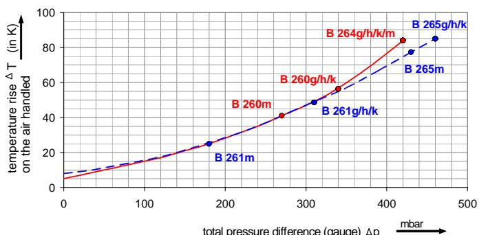
The performance curves are based on air at a temperature of 15 °C and an atmospheric pressure of 1013 mbar with a tolerance of +/- 10 %.
