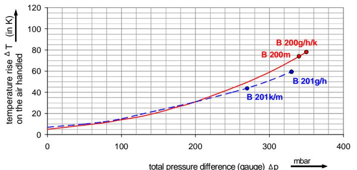
The performance curves are based on air at a temperature of 15 °C and an atmospheric pressure of 1013 mbar with a tolerance of +/- 10 %. The total pressure differences are valid for suction and ambient temperatures up to 25 °C. For other conditions please confer with us.
