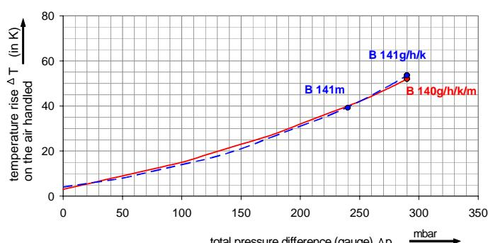
The performance curves are based on air at a temperature of 15 °C and an atmospheric pressure of 1013 mbar with a tolerance of +/- 10 %.
