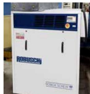
One of the European leaders in the production of disposable plastic tableware and food containers, collaborating with leading international distribution chains too, replaced old vacuum technology with the Robox Screw in vacuum operation. The unit is working at 300 mbar(a) with a consistent energy savings (up to 30kW/h comparing to the previous technology).
