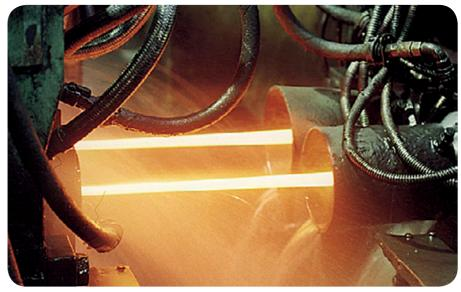
... After rolling, the wire must be cooled quickly. To achieve this, cooling water is sprayed on the wire at a defined pressure and then blown off. As the compressed air comes into contact with the end product, the surface of which must be oil-free, we therefore need oil-free compressed air."
