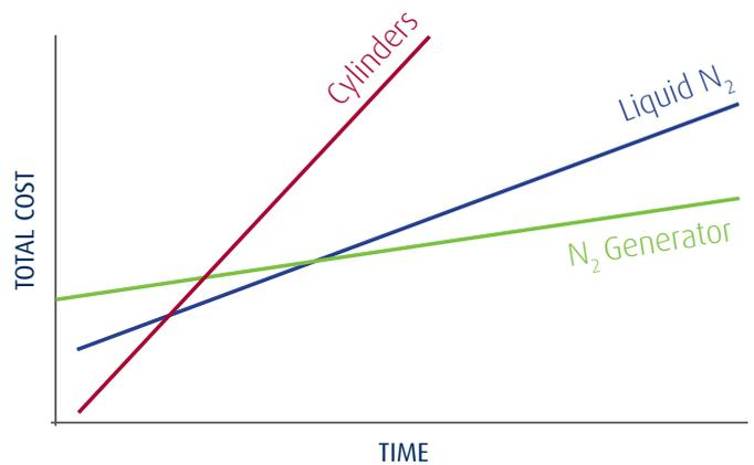
The payback period can be less than one year, when compared to cylinder supply and two to three years, when compared to liquid nitrogen supply.
