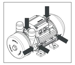
Fig. 5: Points for measuring the vibration speed
