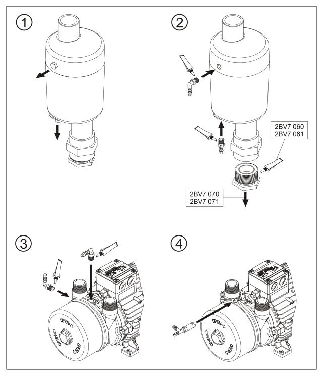
Fig. 20: Mounting liquid separator, Part 1 of 2
