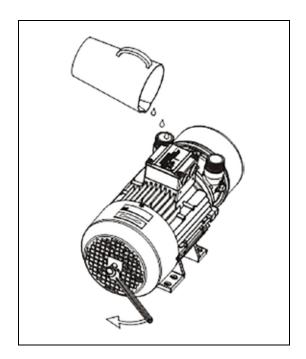
Fig. 16: Pouring in decalcifying agent and freeing shaft by turning
