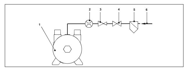
Fig. 11: Operation with operating-liquid feed: Non-automatic operation
