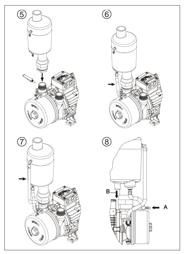
Fig. 21: Mounting liquid separator, Part 2 of 2
