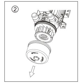
Fig. 15: Removing vacuum pump/compressor housing
