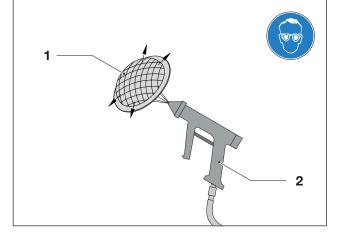
Fig. 6 Blowing out the mesh filter
