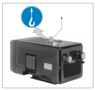
Fig. 1 Lifting and transporting
