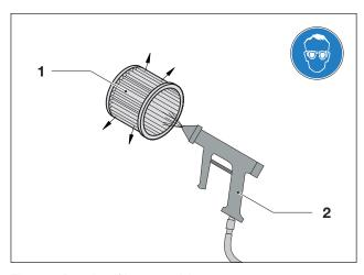
Fig. 6 Purging filter cartridge
