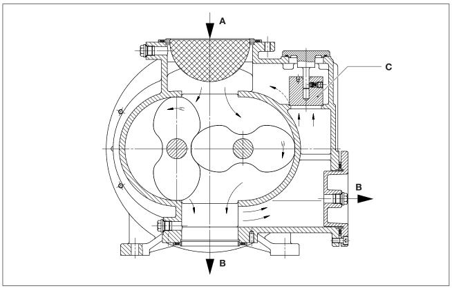
Fig. 5 Rotary lobe vacuum pump R-VWP
