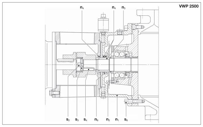
Fig. 13 Changing of the shaft sealing rings and the shaft wearing sleeve VWP 2500
